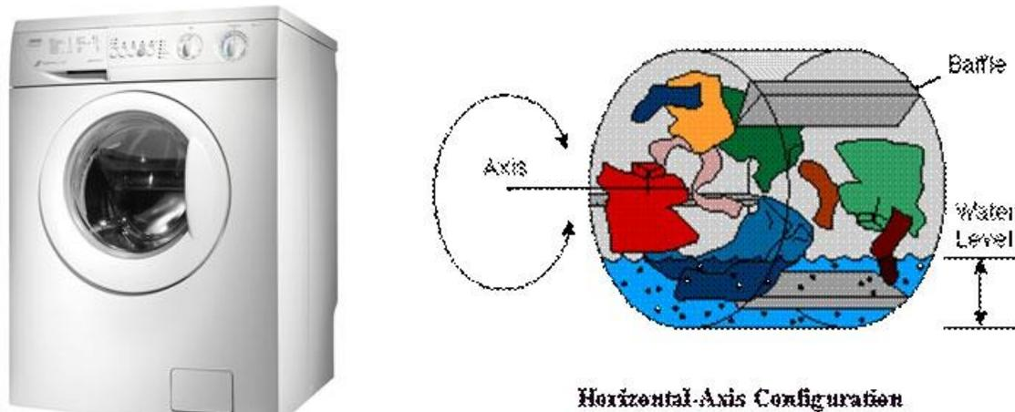
**Caption:** The horizontal-axis configuration of a front-loading washer requires far less water per load than the vertical-axis design of a top-loading washing machine.
