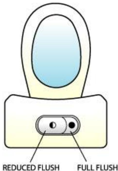
**Caption:** Dual flush toilets conserve water by using the minimum amount necessary for the type of waste.
