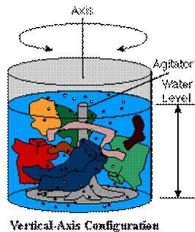
**Caption:** A top-loading washer has a vertical-axis configuration that requires sizable quantities of water to clean clothes.
